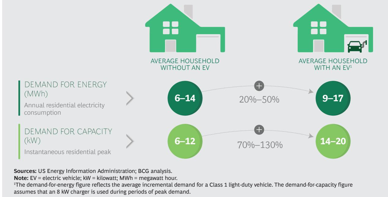
tomers, providing them with a free smart EV charger that automatically shifts charging to periods of low overall demand on the grid.
